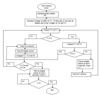
Fig 5: The detailed algorithm of control circuit
