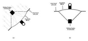
Fig 1: Design of the proposed solar model (a)Stirling engine during day(b) Stirling engine after sun set
