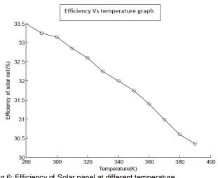
Fig 6: Efficiency of Solar panel at different temperature
